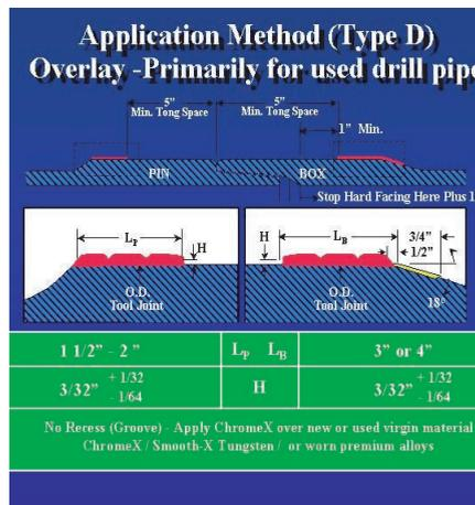
Apply a  $3/32$ -in. thickness (+/-  $1/32$  in.) by 3-in. long raised hardbanding on the tool joint box OD. Start the hardbanding  $1/4$  in. from the taper to allow elevator clearance. Apply a  $3/32$ -in. thickness (+/-  $1/32$  in.) by 1 $1/2$ -in. to 2-in. long raised application to the tool joint pin.
