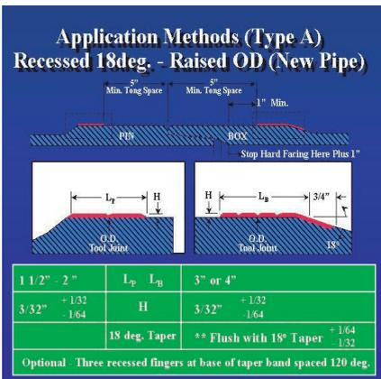
Apply a  $3/32$ -in. thickness (+ $1/32$  in./- $1/64$  in.) by 3-in. long raised hardbanding on the tool joint box OD, tied in to the 18 degree band.
