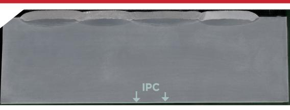
Tool Joints: In addition to lasting longer, there is no damage to IPC due to shallow HAZ
